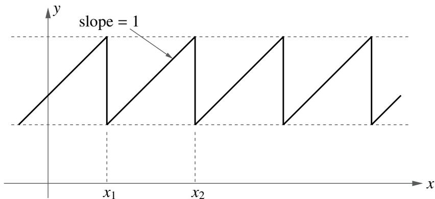
modulo.xbe uses the remainder function to restrict the output y between  $x_1$  and  $x_2$ , as shown in the figure.
