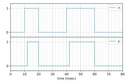
Figure 1: Input x(t) and output y(t) for edge\_delay\_1.xbe. The parameter values are t\_delay = 2m, t\_rise = 0.01m, x\_high = 1.
